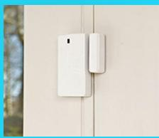
Door sensor will detect if the door/window is opened by someone and send commands to Bahaadur and SMS/call will be activated.
